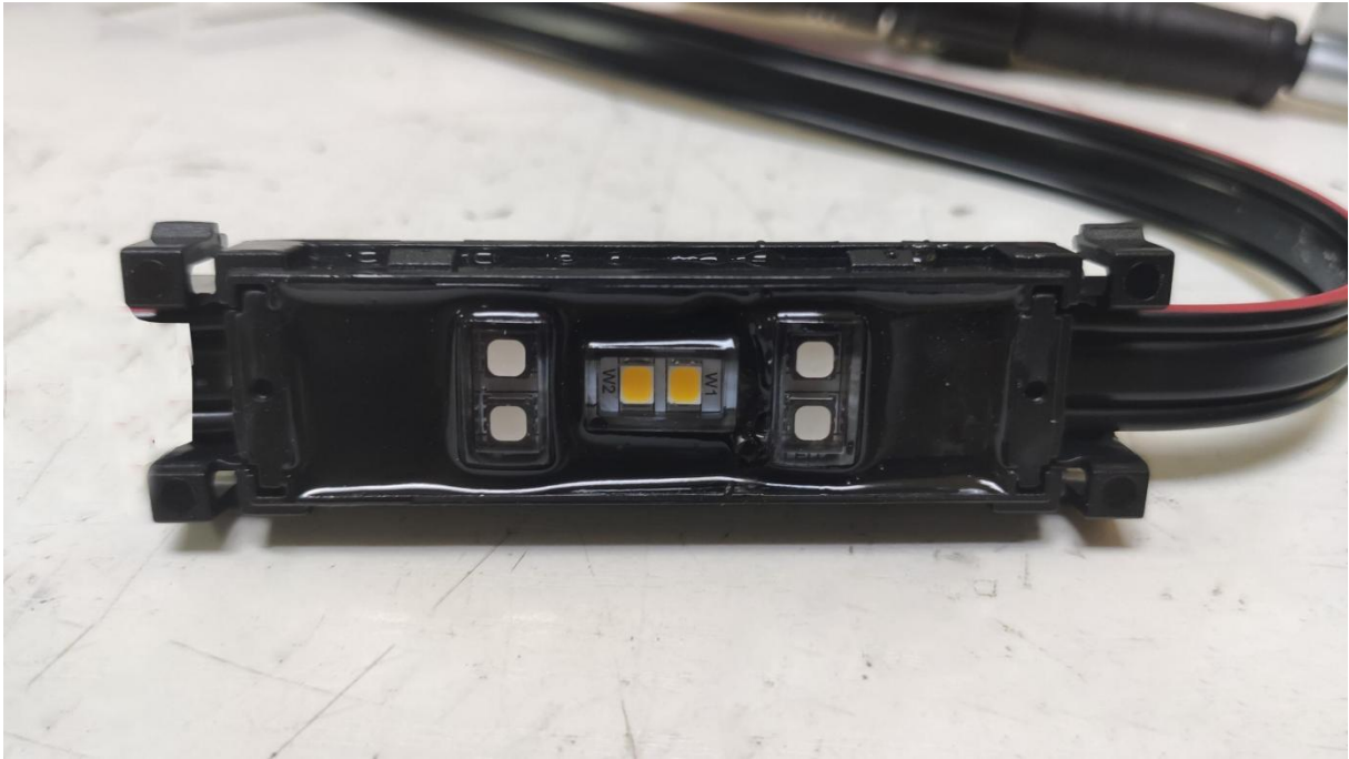
Photo 5: Test result of IP6X and IPX6 test
