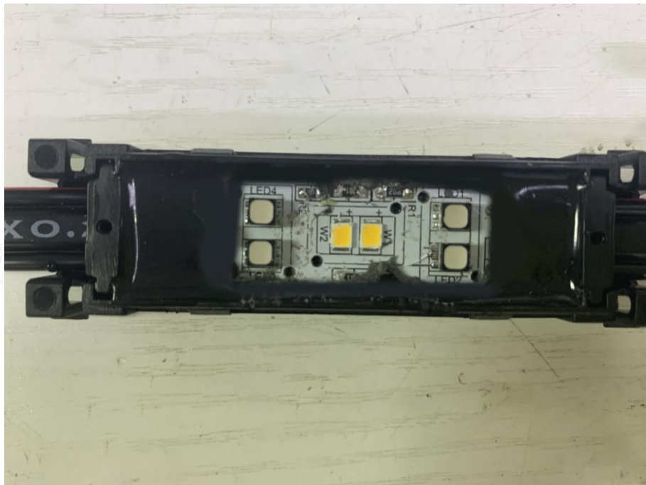
Photo 6: Test result of IP6X and IPX6 test
