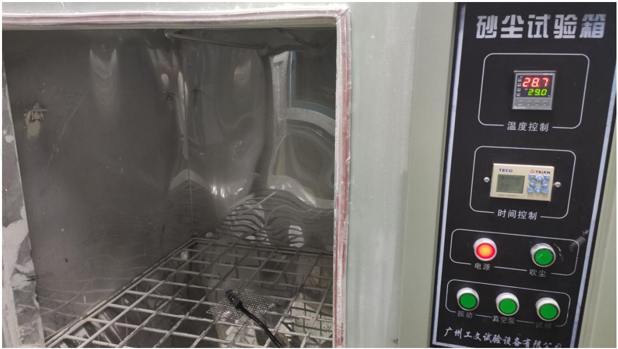
Photo 3: IP6X test of model PP0003-LED1.8M-RGBW-85D
