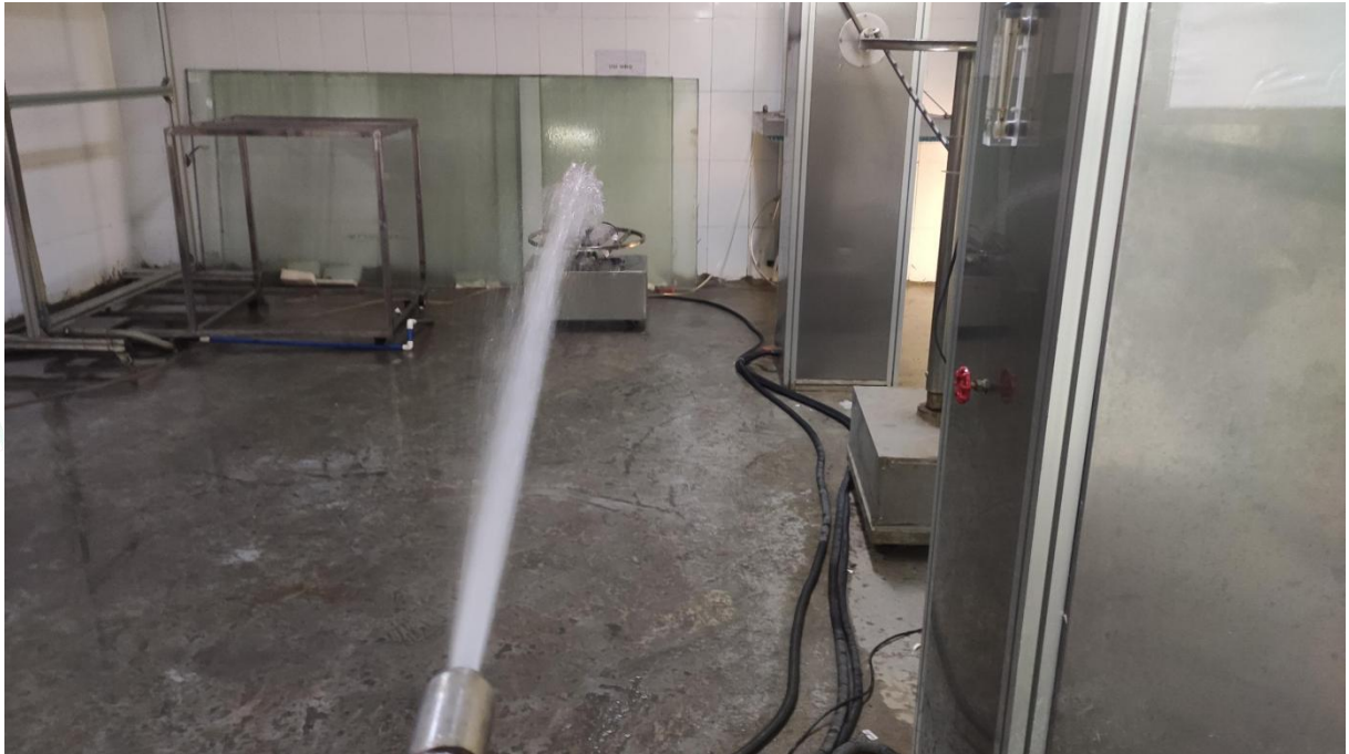
Photo 4: IPX6 test of model IPP0003-LED1.8M-RGBW-85D
