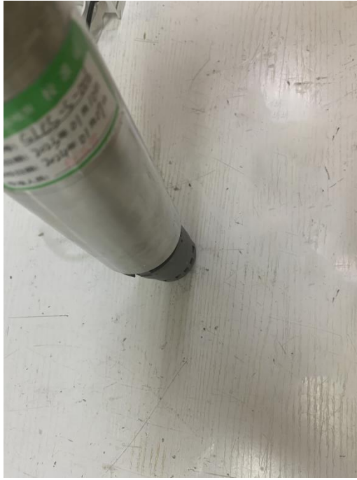
Photo 3: IK03 test of model IS0002-LED07-3090-36D
