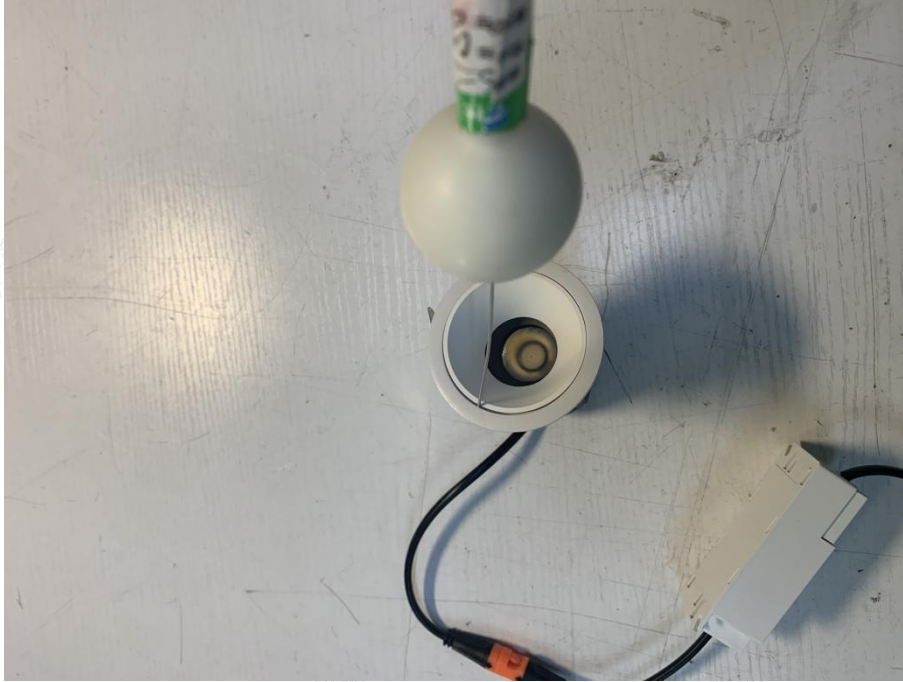
Photo 3: IP4X test of model IS0002-LED07-3090-36D
