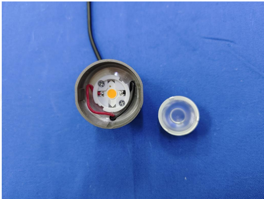
Photo 6: Test result of IP4X and IPX4 test
