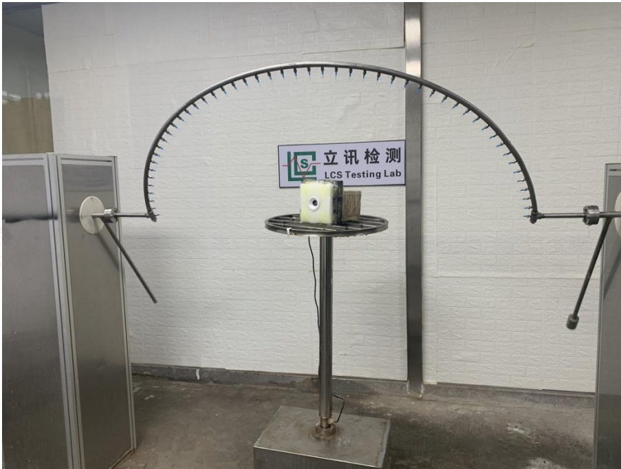
Photo 4: IPX4 test of model IS0002-LED07-3090-36D
